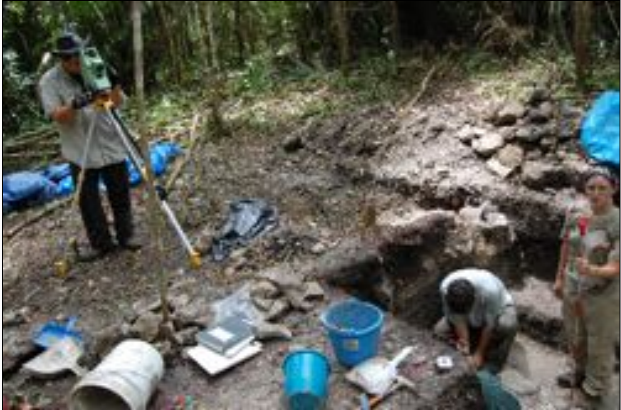
Figure 1. Surveyors Greg Hansen and Brittan Burrell use a Total Station to survey Sub-Structure B-2 in Plaza B at Pacbitun.
